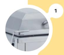
Stainless steel construction makes Multivac chamber machines particularly sturdy and robust. This makes them ideal for constant use in professional environments with high-volume demand. It is also a major advantage in terms of hygiene as the machine is very easy to clean.
