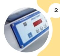
Every Multivac chamber machine is equipped with an electronic control unit that functions as the brain of the system. This ensures optimal packaging with a perfected automatic program and provides a total of six memory positions. Each system is also built with a gentle ventilation system and vacuum sensor to help prevent punctures.
