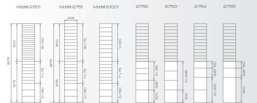
Examples of locker rows consisting of the eight standard locker sizes of the total range
